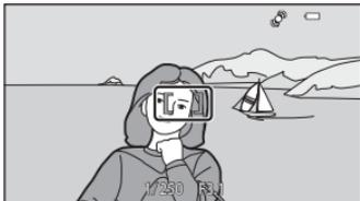
**3** Continue holding down the shutter-release button halfway and recompose the picture.
