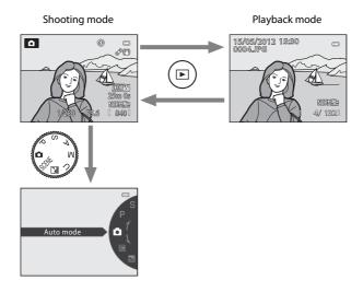
Rotate the mode dial and align an icon to the mark to select different shooting modes (□24, 25).
