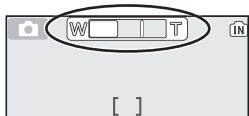
Indicator in monitor shows amount of zoom when either button is pressed
