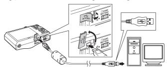
The camera is automatically turned on and the power-on lamp will light. The camera monitor will remain off.
